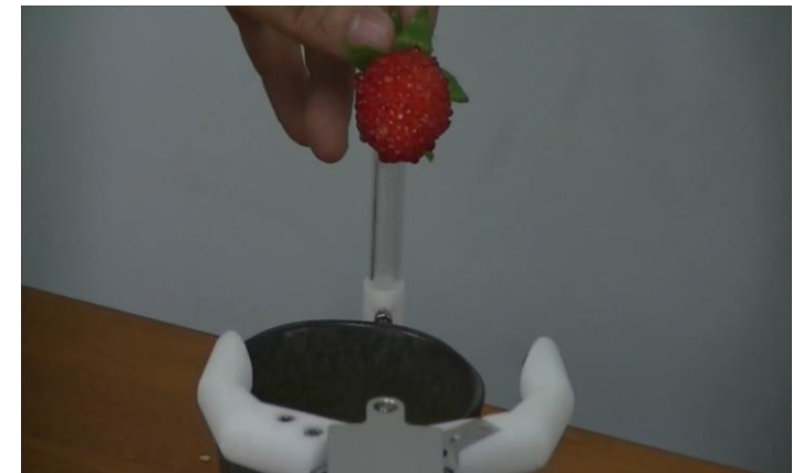
adaptive motion for variation of grasping target (strawberry, thin cookie, plastic cap)
