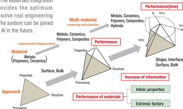
Materials Integration uses all scientific knowledge to help research and development of materials and structures. The system is designed from an engineering point of view. The system also provides information on the effect of service environment on the performance of materials and components. These computer-based estimations help to save research and development time.
