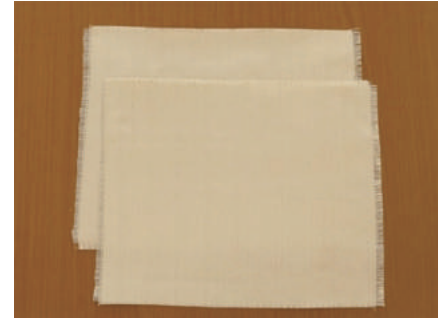
Woven fabric of continuous alumina
