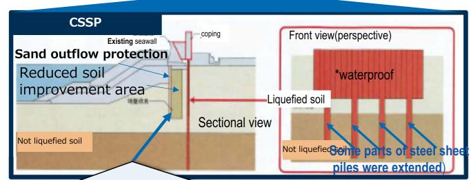
As a result of applying the proposed SIP liquefaction measures package and the large-scale shake table test result, the CSSP showed good performance.
