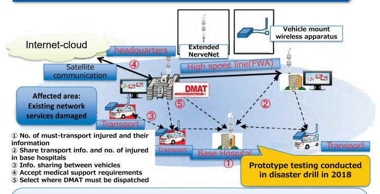
■ Even in areas where existing network services are damaged, patient information during transport can be shared by combining the developed extended Nerve-Net, a kind of long-distance wireless node, with high-speed lines such as FWA.
