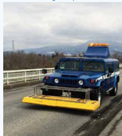
Detection of deteriorated portions inside a floor slab using an onboard high speed scan radar
