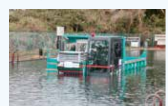
Transport robot for unmanned construction in the semi-submerged environment
