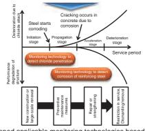
Mapped applicable monitoring technologies based on the progress of deterioration.
