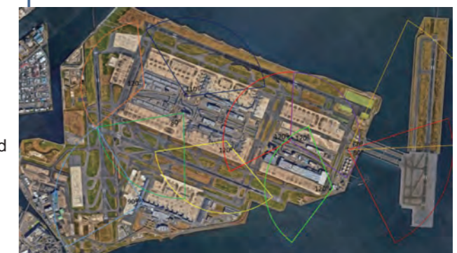
GB-SAR arrangements to cover all the area of Haneda airport
