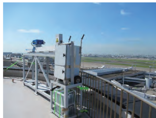
GB-SAR system installed at Haneda airport
