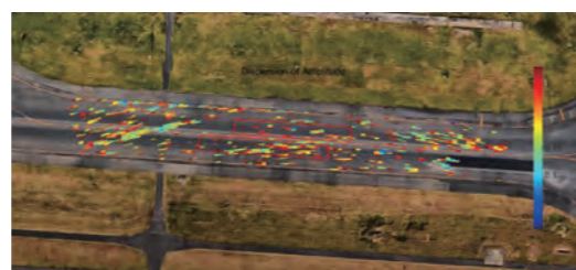
Interferometric SAR image of the pavement surface obtained at Haneda airport
