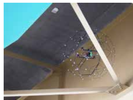
UAV inspecting inner bridge structure (Diameter: 0.95 m, weight: 2.5 kg)
