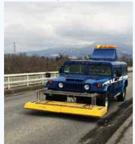
Detection of deteriorated portions inside a floor slab using an onboard high speed scan radar
