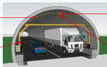
Deformed frame inspection system that does not hinder the transportation
