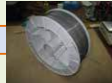
Wire for thermal spraying of Al-Mg-Ca alloy
