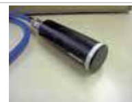
Magnetic probe for corrosion detection
