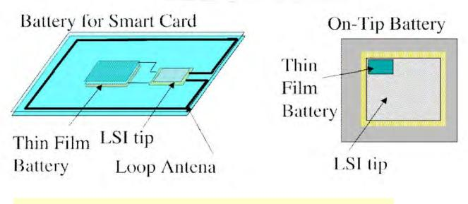
Possible application of thin film lithium batteries
