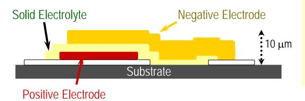
Thin film lithium batteries will be used in things like smart cards, RFID tags, and other low power portable devices.
