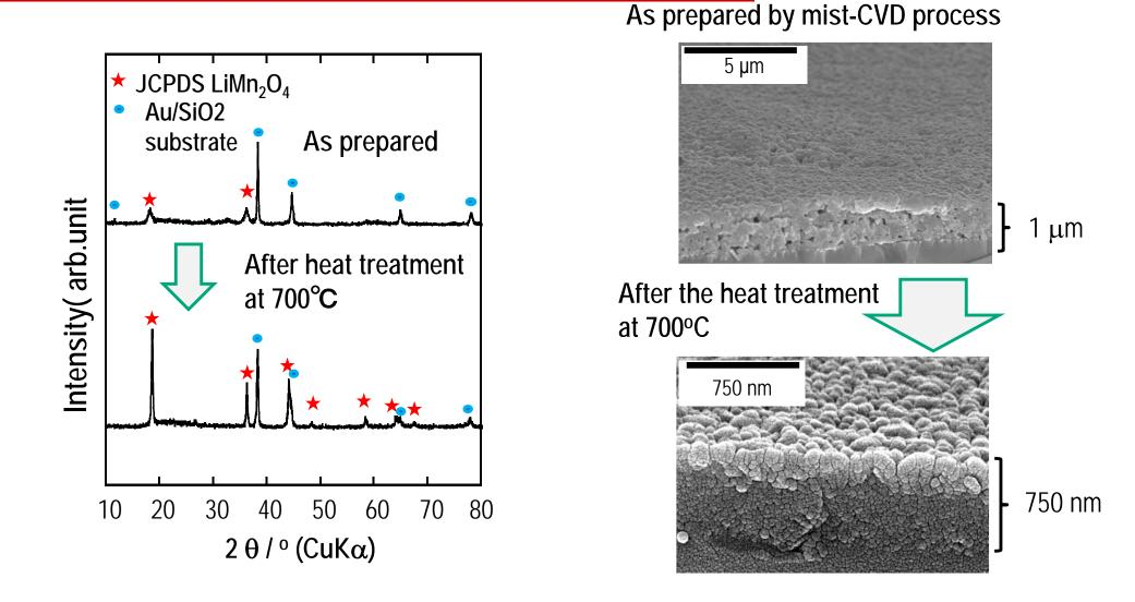
Spinel type  $LiMn_2O_4$  single-phase thin film was obtained.
