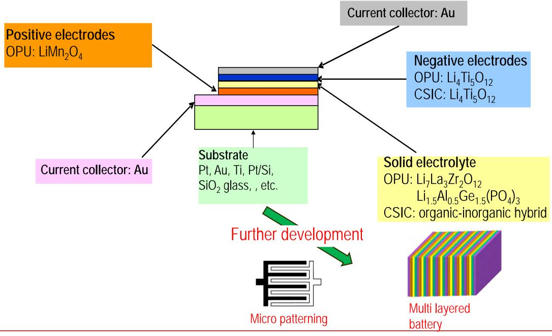
Solution-based processes used in OPU, for the preparation of electrode and electrolyte thin films
