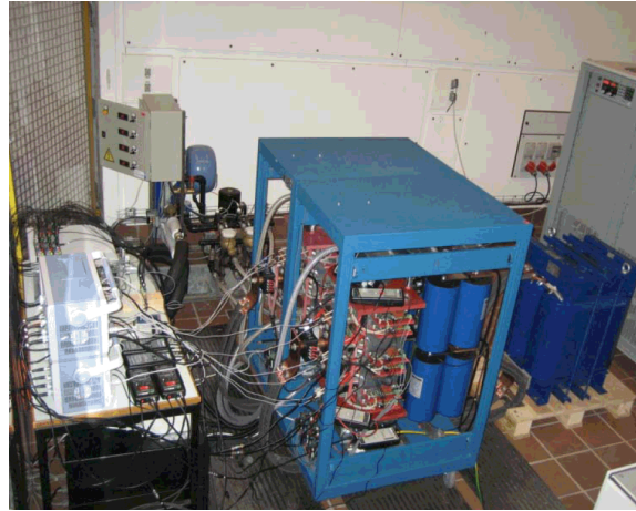
MV lab for testing 6MW 3.3 kV converter
