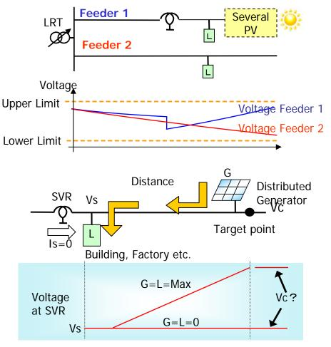
SVR (SVC) can detect only voltage at its location. Voltage at Target point can be strongly
