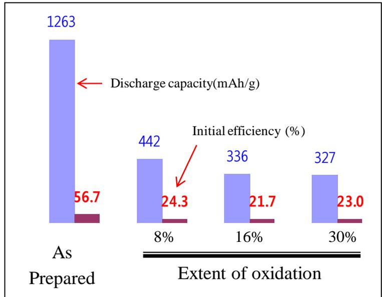
Adhesive power and uniformity of CNF was improved by surface oxidized Si, where as charge-discharge performance became poor.
