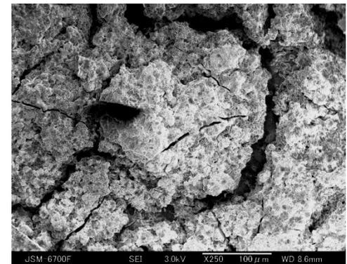
Large crack was observed by cycles
