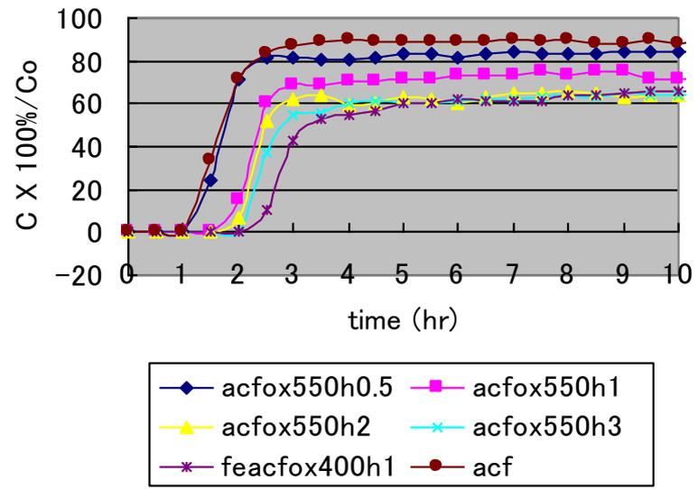
SO2 = 1000ppm, acf = 100 mg. All samples were heat treated at 1100°C
