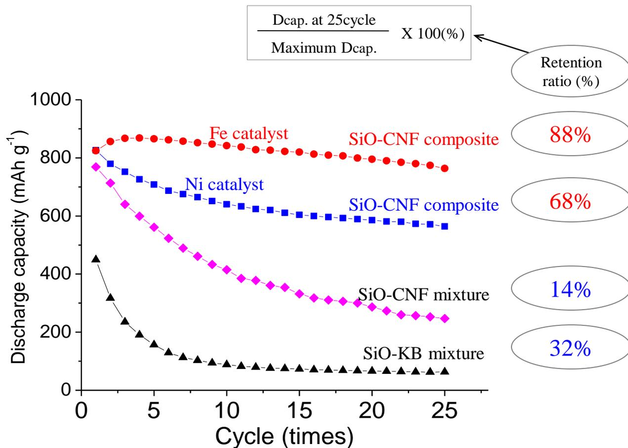
**SiO-CNF composite showed the better discharge capacity, cycle performance and retention ratio than mixtures.**
