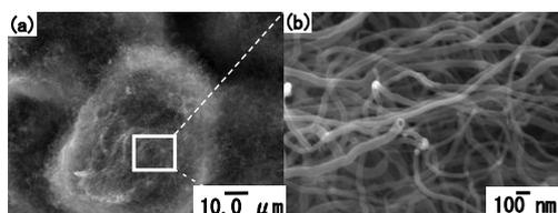
Fig. 1 SEM images of grown Dia.-CNFs from Ni (5 wt%)/O-dia catalyst. Dia.-CNFs were grown at 550 °C by CVD using methane as a carbon source.
