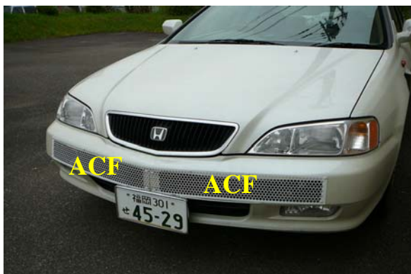
Photo. 2 ACF purification system installed in vehicle
