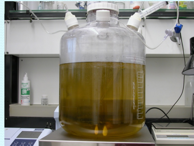
liquid culture in fermenter (5 L scale)
