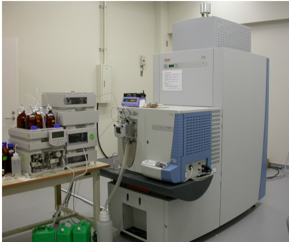
LTQ-FT (Thermo Electron Co.) Magnetic field: 7 T
