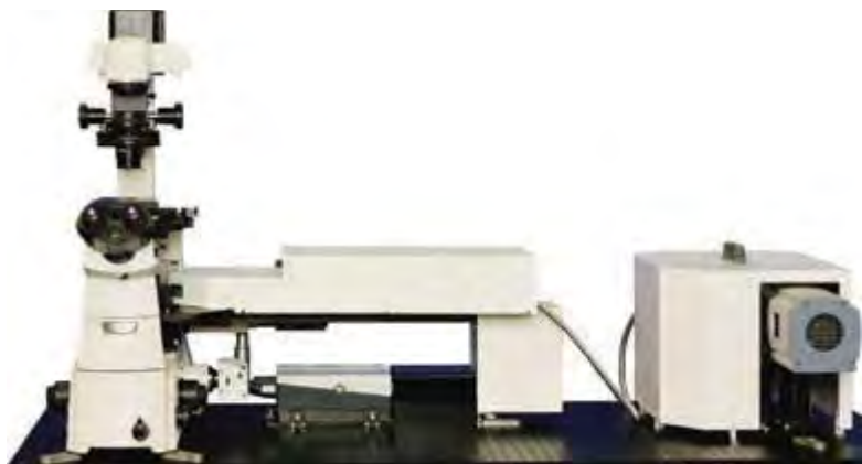
Fig. 1 Appearance of inverted-type two-dimensional multi-point confocal Raman microscope. The left unit consists of an optical microscope, a multi-point confocal optic unit, and an excitation laser. The right one consists of a transmission-grating spectrograph and a CCD detector. The two units are linked with a fiber bundle.
