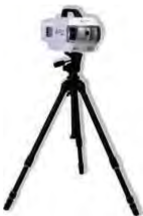
Fig. 1 Photograph of ASTROCAM 7000 HS. The Si/CdTe Compton camera and an optical fish-eye camera are included.
