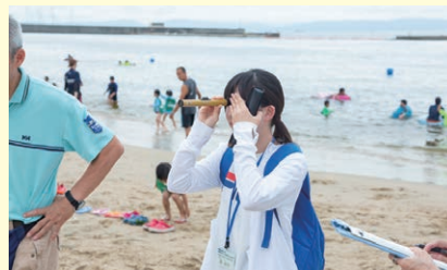
(1) Decide the investigation spot and measure and record distance from and height disparity with the beach edge.
