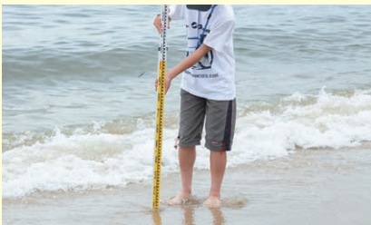
(1) Decide the investigation spot and measure and record distance from and height disparity with the beach edge.
