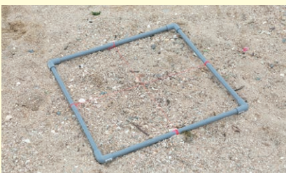
(2) Collect sand to a depth of about seven centimeters within a space of 50 square centimeters indicated by the frame.
