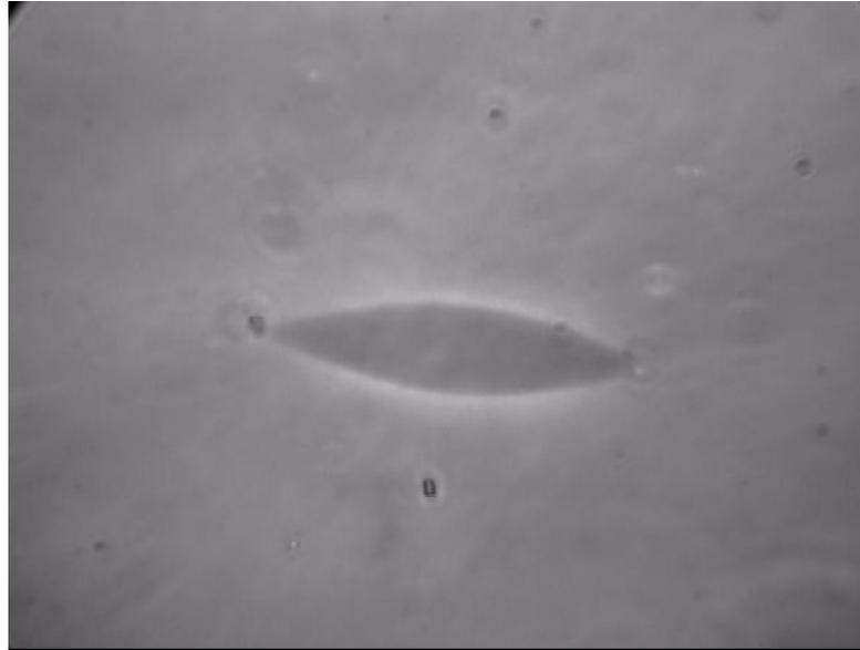
The amoeba-type molecular robot changes its shape by **light irradiation**, accompanied with **stretching and shrinking** of filopodia-like extensions.
