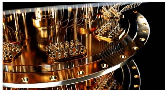
A section of a quantum computer based on superconductors. Researchers at NEC are exploring such quantum computers. Credit: Bartłomiej Wroblewski/iStock/Getty
