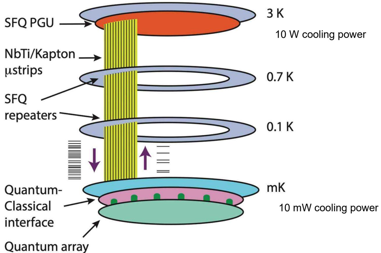
Quantum layer = qubits and readout resonators only; minimal fab processing
