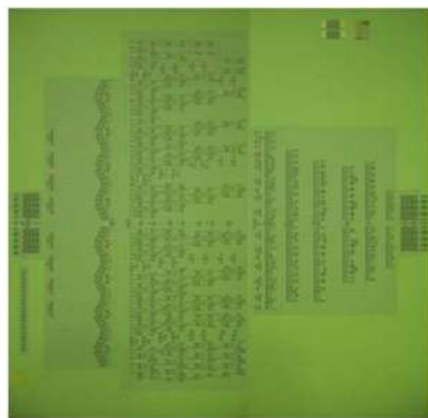
48-GHz 8-bit Multiplier 20,251 JJs I. Nagaoka, ISSCC 2019
