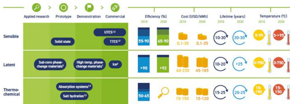
Fig. II-23: Progress in the development of heat storage materials for regional heating and cooling systems and development goals for 2030 (Reference: IRENA, Innovation Outlook Thermal Energy Storage, 2020)
