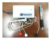
A prototype device was created to improve the accuracy of heart rate and autonomic nerve measurement in daily life and to enable long-term measurement.
