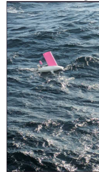
Fig. 3 VM drone prototype No. 3, deployed during R/V Mirai western North Pacific/Bering Sea cruise for weather resistance test under typhoon-level stormy conditions.
