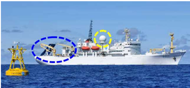
Fig. 1 R/V Mirai used for open-ocean tests of prototypes. A-frame crane on the aft deck (blue dashed circle) and other equipment used for deployment and retrieval of the VM drone prototypes. C-band radar (yellow dashed circle) and various atmosphere-ocean sensors equipped with the vessel are used to validate data obtained by the prototypes.
