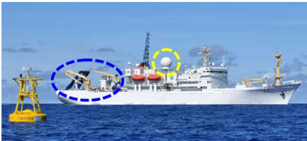
Fig. 1 R/V Mirai used for open-ocean tests of prototypes. A-frame crane on the aft deck (blue dashed circle) and other equipment used for deployment and retrieval of the VM drone prototypes. C-band radar (yellow dashed circle) and various atmosphere-ocean sensors equipped with the vessel are used to validate data obtained by the prototypes.
