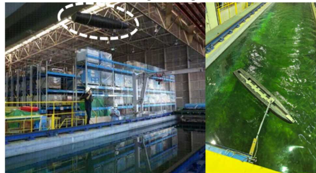
Fig. 2 Water tank tests using VM drone prototype #0. It was lifted up to the ceiling by a crane (white dashed circle) and dropped into the water tank for a strength test (left). The prototype #0 with six-axis stress sensor equipped to its mast was towed at high speed over the water tank to measure wave resistance and stress around the mast (right).
