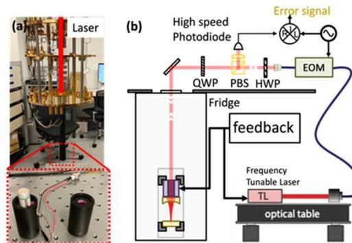
Figure 2 Stabilizing an optical cavity in a dilution refrigerator. (a) Photographs of the custom dilution refrigerator (top) and the cavity (bottom). (b) Schematic of the setup.
