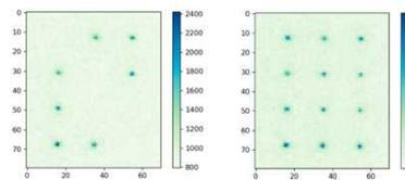
Fig. 2: CCD image of demonstrated atomic array.
