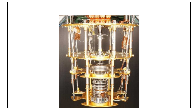
Dilution refrigerator under prototype
