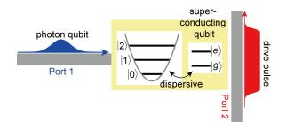
exchange (SWAP gate) between a superconducting qubit and a microwave-photon qubit and demonstrated it in collaboration with an experimental group. The proposed gate can be easily operated by simply reflecting photon qubits onto the superconducting qubits. The average fidelity of photon to atom (atom to photon) state transfer reached 0.829 (0.801). This value can be further improved by extending the qubit lifetime.
