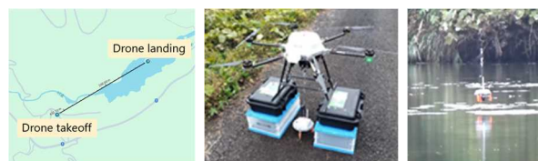
Figure 4: Drone takeoff/landing site (left), the drone carrying the sensor device (center), the device just before water landing during autonomous transport (right).
