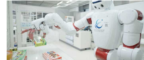
Figure 3: Object grasping verification in a convenience store environment using Dry-AIREC
