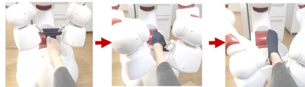
Fig.2 Putting-on socks motion by Dry-AIREC
