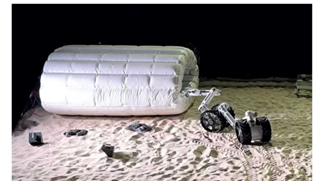
MoonBot-Assisted deployment of HIDAS (inflatable structure)
