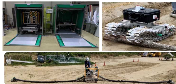
Figure 9: An overview of the modular transport container “BRAINS” that enables separation and recombination (top left), a mobile unit to traverse challenging terrain (top right), and the working unit designed for hose deployment (bottom).
