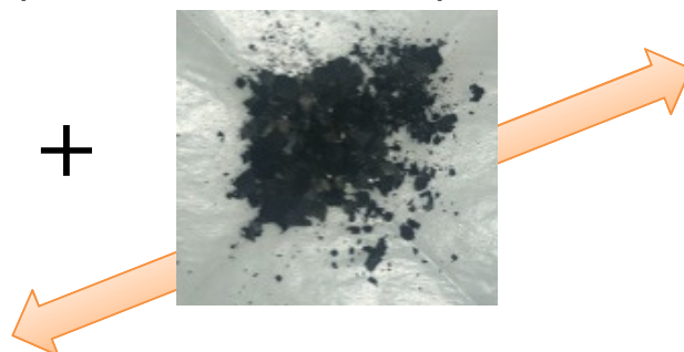
Separated positive electrode particles
