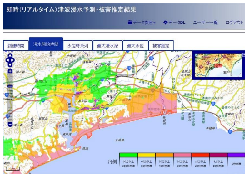
Figure A2-19. Output of the real-time tsunami damage forecast system (e.g., inundation start time)
