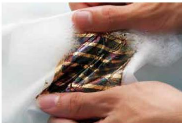
Figure A2-12. Washing of ultra-thin organic solar cells attached to clothes
