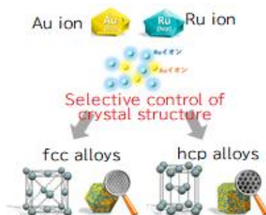
Figure A2-13. An innovative method to control the crystal structure of nano-alloys
