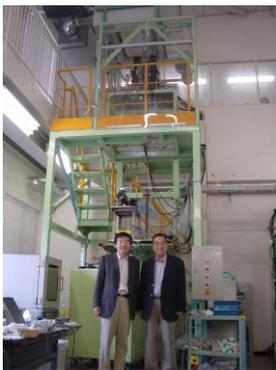
Figure 1 Appearance of co-extruder for preparing GI-POF.
