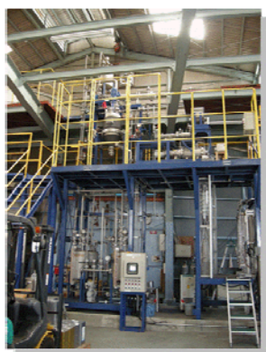
Fig. 1 Continuous system plant for refining lignocellulosics into lignophenols and carbohydrates.
