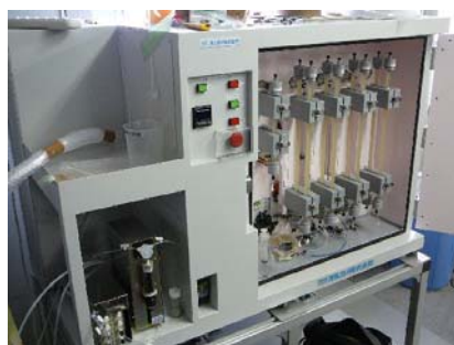
Fig. 6 Apparatus for separation of carbohydrates and sulfuric acid.
