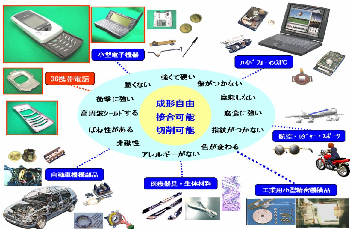
Fig. 28 Properties of bulk metallic glasses and their applied products.
