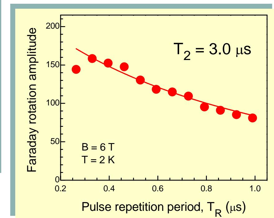
decay time gives single dot coherence time  $T_2 = 3.0 \mu\text{s}$
