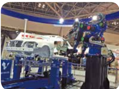
▲ MOTOMAN-VS100 is a spot welding robot used in automobile production. (Yaskawa Electric Corporation)
