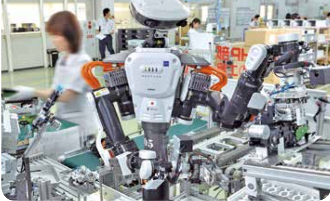
▲ NEXTAGE works in tandem with human workers on factory assembly lines. (Kawada Robotics)
