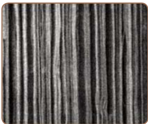
Structure of copper alloy based on this technology (filament reinforcement)
