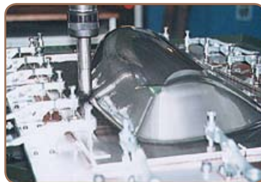
Dieless forming machine (working space)
