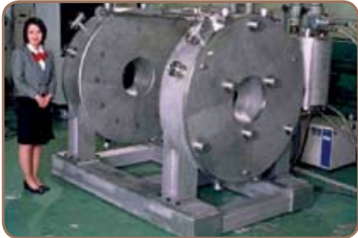
High-temperature superconducting magnet for Si single-crystal grower
