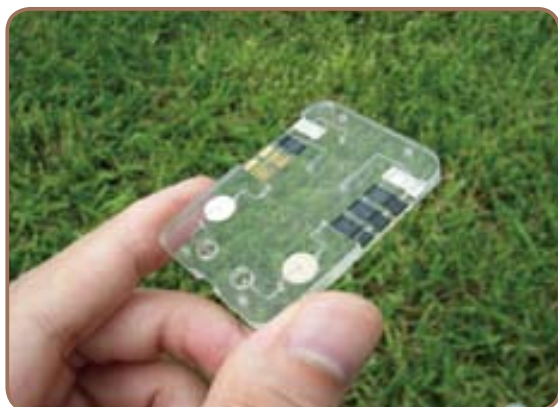
Minute electrochemical cell (sensor chip)
