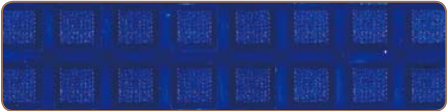
Sample of measurement (approximately 2000 DNAs are identified per spot)
