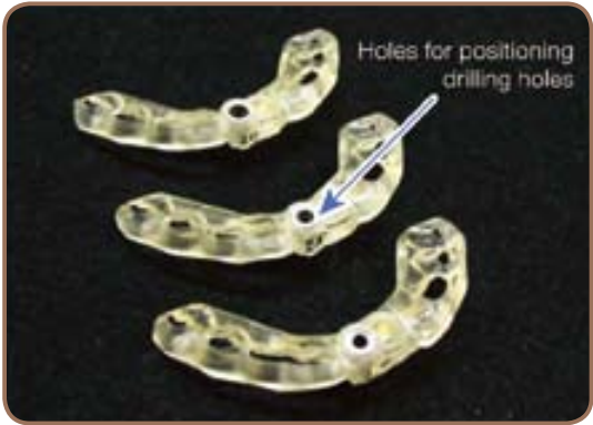
Surgical guide molded using 3D resin lamination molding machine
