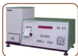
Oil deterioration measuring instrument (under development) Chemiluminescence analyzer OX-7 (standard type)
