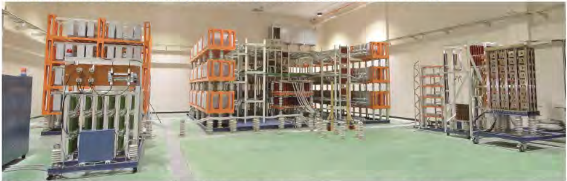
Lightning resistance evaluation equipment (B/C generator)
