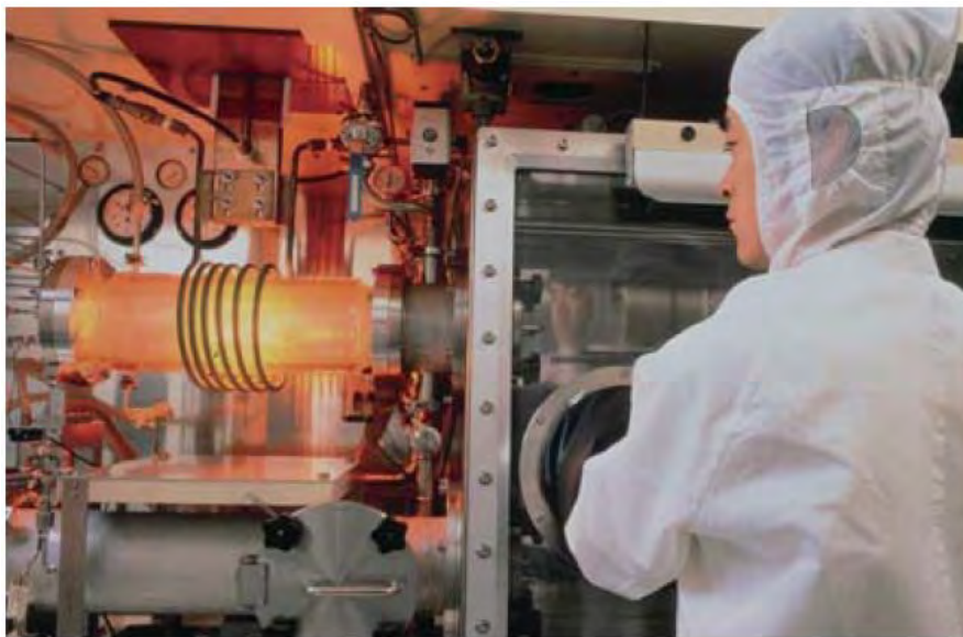
Experimental devise for GaN crystal growth in 1987
