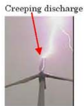
Pic2. Creeping discharge
