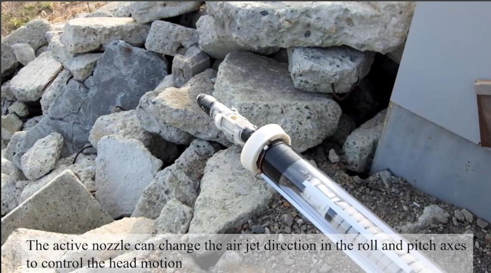
The active nozzle can change the air jet direction in the roll and pitch axes to control the head motion
