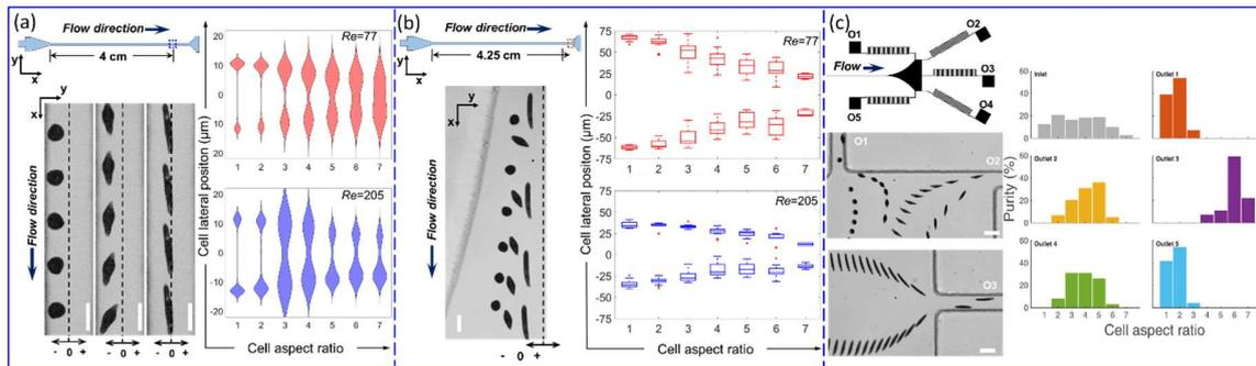
Figure 2 Shape-activated differences in lateral positions of *E. gracilis* cells with different aspect ratios ranging from 1 to 7 at a straight region 4 cm downstream from the inlet (a), an expansion region (b), and the collection outlets (c). High aspect ratio cells,  $AR>4$  are enriched in outlet 3, while lower aspect ratio cells,  $AR<4$  are enrichment in outlets 1 and 5, as can be seen in the histograms of the collected cells.
