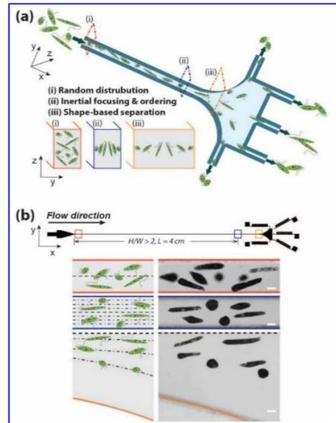
Figure 1 Schematic (a) and experimental (b) illustration of the device design and sorting principles for shape-based algae sorting.
