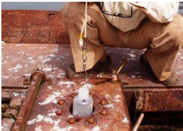
図7. Checking the diameter of a degassing pipe at Lake Monoun.
