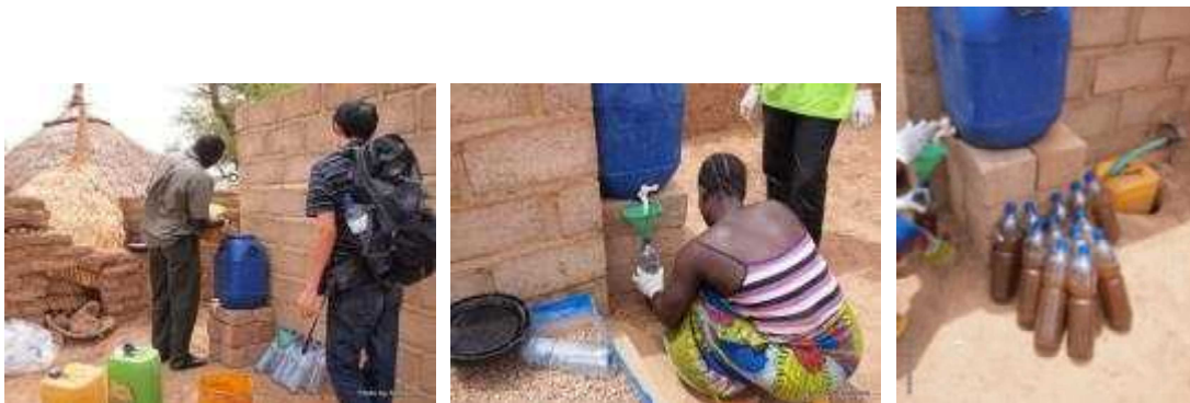
Fig.7 Another urine tank, urine transfer, and solar disinfection.
