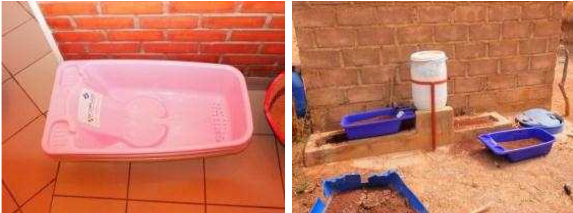
Fig.4 first soil chamber modified from baby bath
