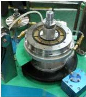
A new portable hand-driven ring shear apparatus under development by the Croatia-Japan Joint project in 2010.
