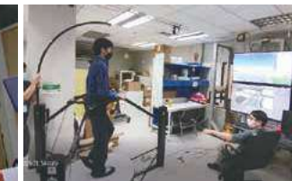
VR-integrated treadmill used to evaluate and improve walkability of street environments
