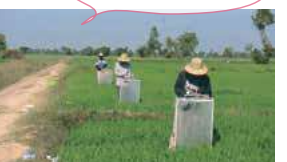
Sampling of paddy field methane emissions using the chamber method
